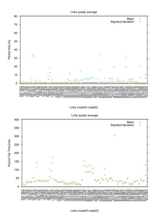
**Figure 4.4:** Average packet loss (top) and RTTs (bottom) of all links of one week long measurement campaign. Parametrisation in Table 3.1.
