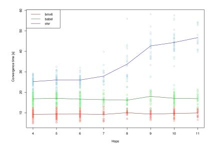
**Figure 4.16:** Convergence time depending on number of intermediate hops. Parametrisation in Table 3.5 and Table 3.6.
