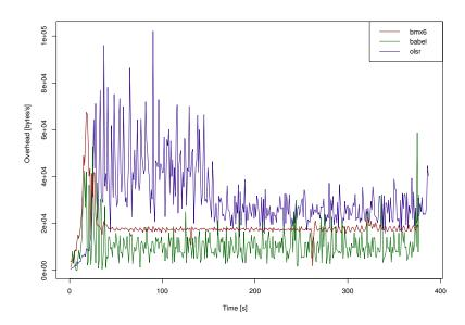
**Figure 4.7:** Protocol overhead of all daemons started in parallel. Integration period: 1s. Parametrisation in Table 3.3.
