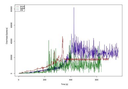
**Figure 4.8:** Protocol overhead of all daemons started in serial. Integration period: 1s. Parametrisation in Table 3.4.
