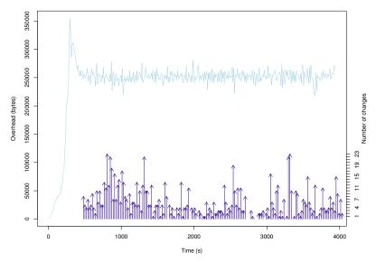
**Figure 4.14:** *OLSR protocol overhead over time affected by discrete link changes. Parametrisation in Table 3.6.*
