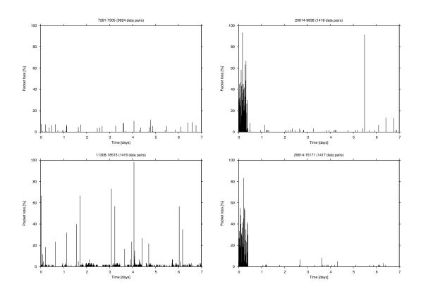
**Figure 4.2:** Packet losses of an excellent link (top left), a poor link (bottom left) and two links of a node affected by interferences during the first half measurement day (top right and bottom right). Parametrisation in Table 3.1.
