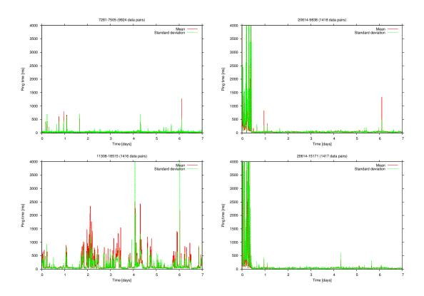
**Figure 4.3:** RTTs of an excellent link (top left), a poor link (bottom left) and two links of node affected by interferences during the first half measurement day (top right and bottom right). Parametrisation in to Table 3.1.
