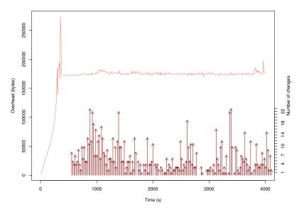
**Figure 4.13:** *BMX6 protocol overhead over time affected by discrete link changes. Parametrisation in Table 3.6.*
