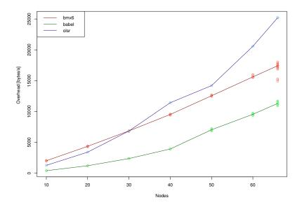
**Figure 4.9:** Protocol overhead of all daemons depending on number of nodes. Parametrisation in Table 3.5.
