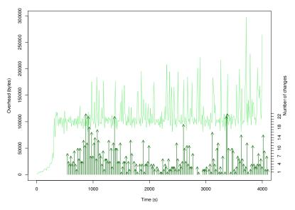
**Figure 4.12:** Babel protocol overhead over time affected by discrete link changes. Parametrisation in Table 3.6.
