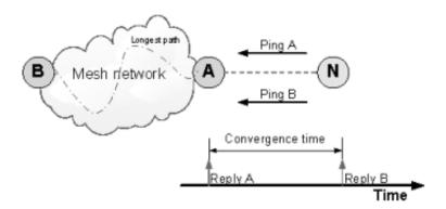
**Figure 3.1:** *Convergence time measurement method.*
