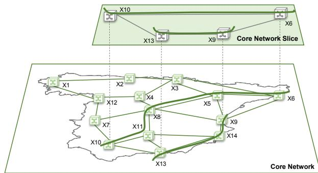
Figure 2. Core network slice physical mapping.
