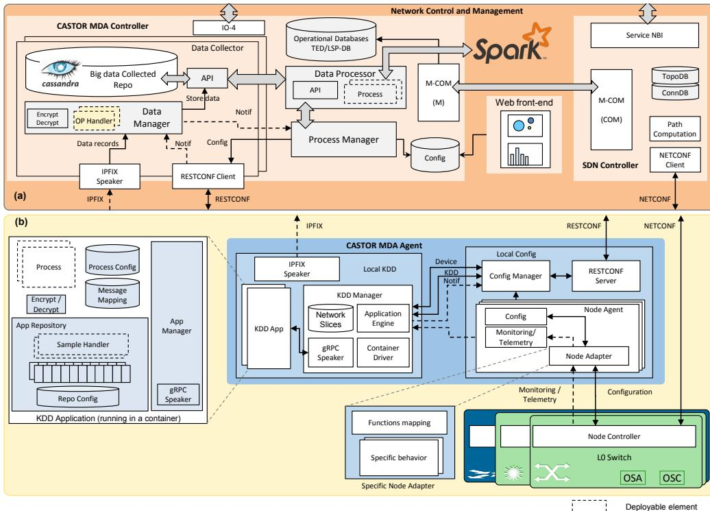
Figure 4. CASTOR architecture details: a) MDA controller and b) MDA agent.
