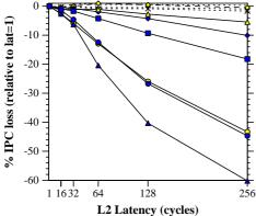
Figure 1-d: Impact of latency on performance.
