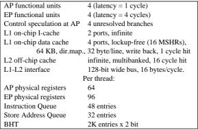
**Figure 2:** Scheme and main parameters of the multithreaded decoupled processor
