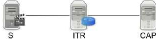
Figure 7: Testbed. S generates CoreCast traffic, ITR processes the packets, and CAP captures the resulting traffic
