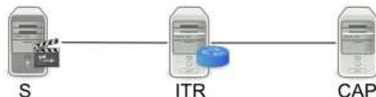
Figure 7.4: Testbed. S generates CoreCast traffic, ITR processes the packets, and CAP captures the resulting traffic
