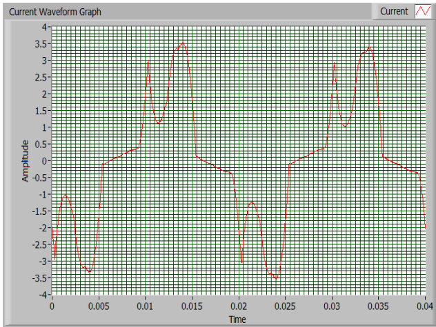
Fig. 10. Current waveform graph of inverter air conditioner, Operation mode: Cooling, Line voltage RMS: 235,14 V, Load current RMS: 1,817 A, THDI: 49,868 %.
