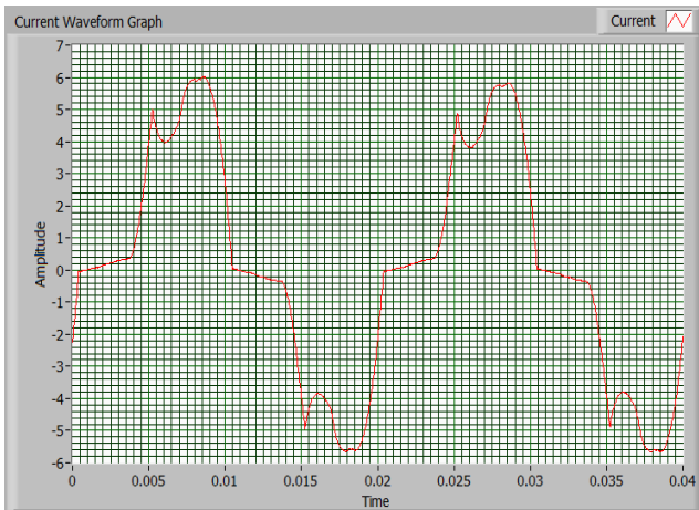
Fig. 11. Current waveform graph of inverter air conditioner, Operation mode: Heating, Line voltage RMS: 233,16 V, Load current RMS: 3,487 A, THDI: 34,368 %.
