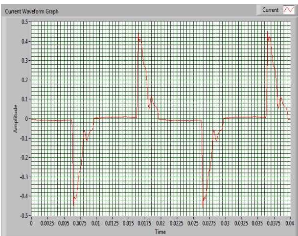
Fig. 8. Current waveform graph of ECO Energy saving light, THDI=113,12\% .
